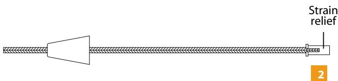
**2** Insert the coaxial cable through the flared end of the strain relief.
