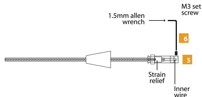
**5** Insert the coax wire into the connector and you'll notice the coaxial braid will start to bulge, while continually inserting the wire into the connector start to slide the strain relief closer into the connector opening until the coaxial wire terminates with its inner wire visible through the TIP of the connector. Meanwhile insert the strain relief inside the connector until it is flush.
