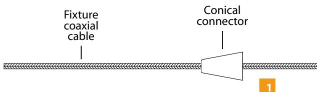
**1** Cut coaxial cable to desired hanging length of the pendant and insert the fixture coaxial cable through the conical connector
