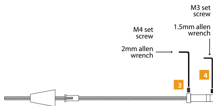
**3** Loosen (Do Not Remove) the M4 set screw with the provided 2mm Allen wrench.
